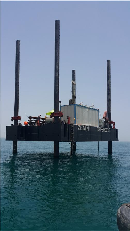
Z Makina specializes spud barges in customized barge manufacturing for use pile driving, crane barge, drilling barge, etc. Barges can be spudded in place (sea or lake) due to its special design and it provides easy application. They differ in size and structural design, depending upon their intended use.
