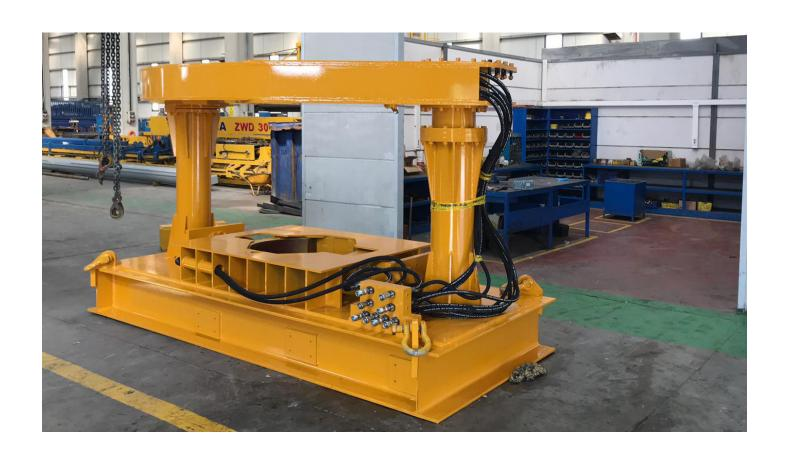
The installation of the conductor casings ranging from 20" to 30" diameter are installed by the Power Tong ZPT 30 with the torque needed to make up the conductor pipes is monitored, and controlled. According to the selected diameter of the casing, PLC system limits the tightening torque in order to avoid structural failures. In other words the make-up torque ratings rely on casing size, grade, metallurgy, weight, and the thread compound friction factor being utilized.
