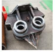
M8 grab was manufactured with the grab jaws for excavation widths 800 / 1000 mm. In addition to the M8 grab Z Makina had
