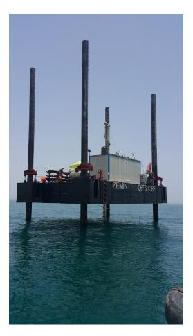
Z Makina specializes spud barges in customized barge manufacturing for use pile driving, crane barge, drilling barge, etc. Barges can be spudded in place (sea or lake) due to its special design and it provides easy application. They differ in size and structural design, depending upon their intended use.
