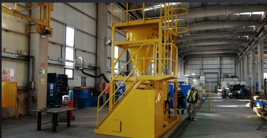
Z Makina Manual Mixers are specially designed for continuous mixing, and very useful in construction areas due to its small dimensions. Mixing time is about 2-3 mins that it can fast mix slurry.
