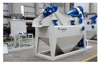
Desander and desilter are solids control equipment with a set of hydro cyclones that separate sand and silt from the drilling mud used on drilling rigs. They can be mounted either sepa-
