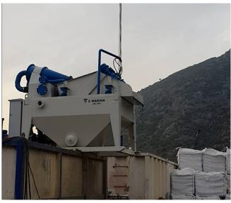
rately or completely. Desander is assembled on top of the mud tank following shale shaker and vacuum degasser, but before the desilter. Desilter is mantled on top of the mud tank following Desander.
