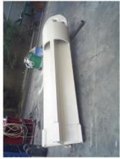
Z MAKINA Diaphragm wall and pile rig chisels penetrate rocks, boulders, and soil limitations to accelerate the grab excavation. Z MAKINA produces a broad selection of chisels in free-fall use to penetrate through the obstructions during excavation. Z MAKINA Chisels incorporate high-tensile, Hardox 500 steel and S 355 on the cutting edges to abrasion for resistance to wear and cold bending.
