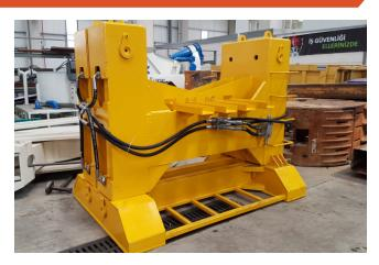
As soon as the concrete begins to set, extractors pull out the stop-end elements. Z MAKINA produces for the extraction of stop-end elements having a width from 500 to 1500 mm and pulling capacity up to 4000 kN. The system is complete with locking system pins to prevent dropping of the column. Z MAKINA supplies the hydraulic power pack for the extractors, customized for the adequate power. A remote control integrated with power pack to operate the unit is also available as optional.
