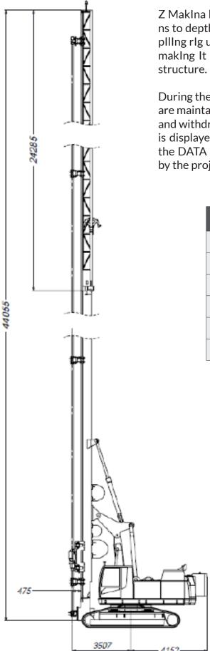
Z Makina has developed a jet grouting system with the single stroke columns to depths of 36 m capacity. It was designed which can be mounted on the pilling rig used for jet grouting come in a range of different sizes; large ones, making it a perfect technique for improving the foundation of an existing structure.
