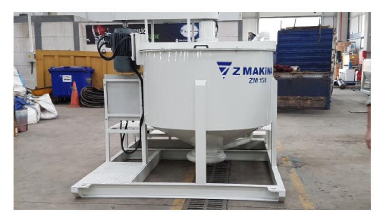
Z MAKINA Manual Mixers are specially designed for continuous mixing, and very useful in construction areas due to its small dimensions. Mixing time is about 2-3 mins that it can fast mix slurry.
