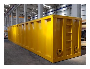
The bentonite tanks for bentonite muds and plastic mixtures are enormously strong that is stiffened oversized profiles, and electro-welded pressed steel sheet with the appropriate thickness.
