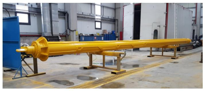
Kelly bar is the main part of a drilling machine, and the performance of the machines is affected by its quality. The fundamental goal of kelly bar is to transfer the maximum torque and pressure supplied by the drilling machine. Z MAKINA provides kelly bar for all types of rotary drilling rigs.
