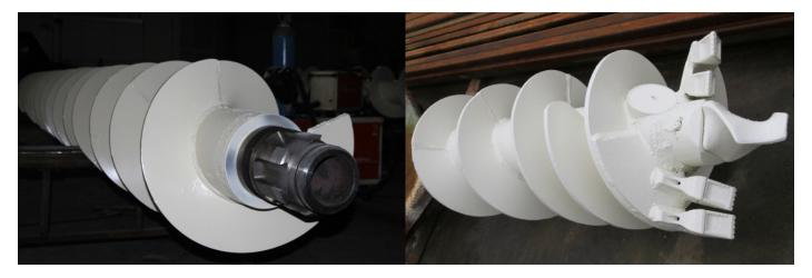
CFA piles are a type of drilled foundation in which the pile is drilled to the final depth in one continuous process using a CFA then concreting through the augers while extracting the tools.
