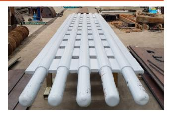
Stop-ends are easily placed to the ground and coupled together through special steel bars. They are made of sheet metal welded and internal pipes reinforcing the structure increasing it strength and toughness to prevent it from any damage. It is easy to connect or disconnect.
