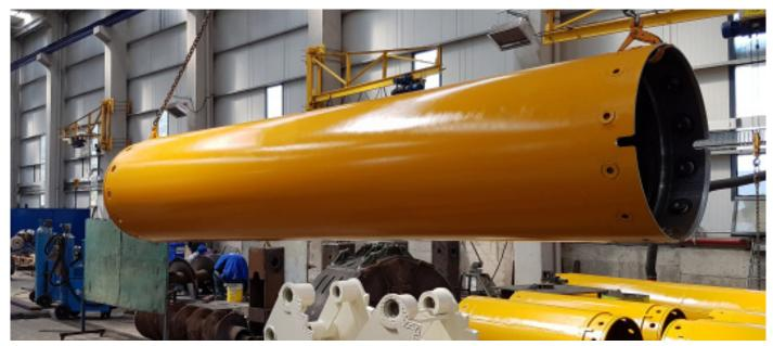
The Casings are used to protect the whole drilling operation; principally the rotary drilling tool during the operation, performs inside a mechanical protection executed by the casings fixed into the ground. Those casings are recovered for reuse.
