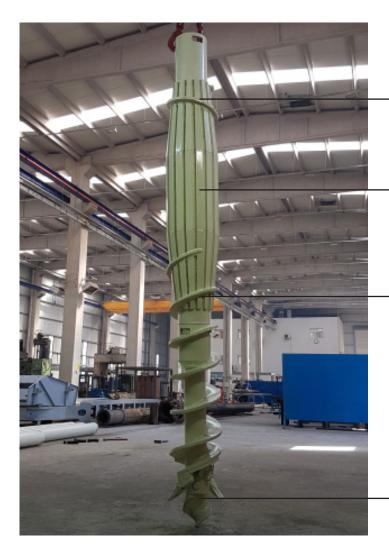
Counter rotating flight body compress the loosened soil while pulling
