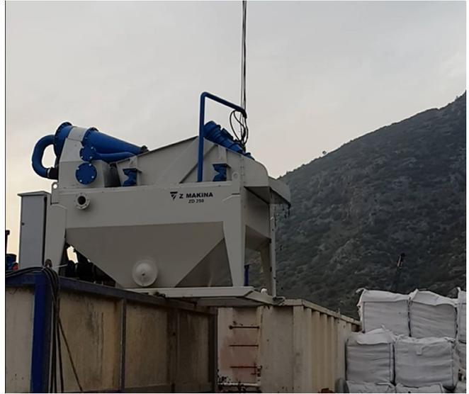
Desander and desilter are solids control equipment with a set of hydro cyclones that separate sand and silt from the drilling mud used on drilling rigs. They can be mounted either separately or completely. Desander is assembled on top of the mud tank following shale shaker and vacuum degasser, but before the desilter. Desilter is mantled on top of the mud tank following Desander.
