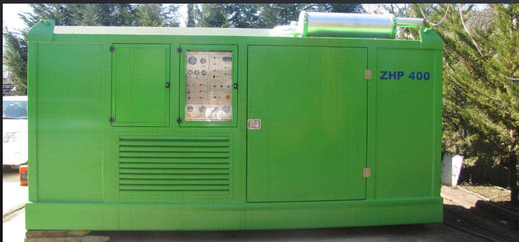
A power pack is a dedicated power source for any application where more hydraulic horse-power is desirable. Z Makina manufactures a wide range of hydraulic power units depending on the variety of applications in soil improvement. The compatible hydraulic system, with variable speed control, provides infinite speed and pump settings for maximum recovery and efficiency.
