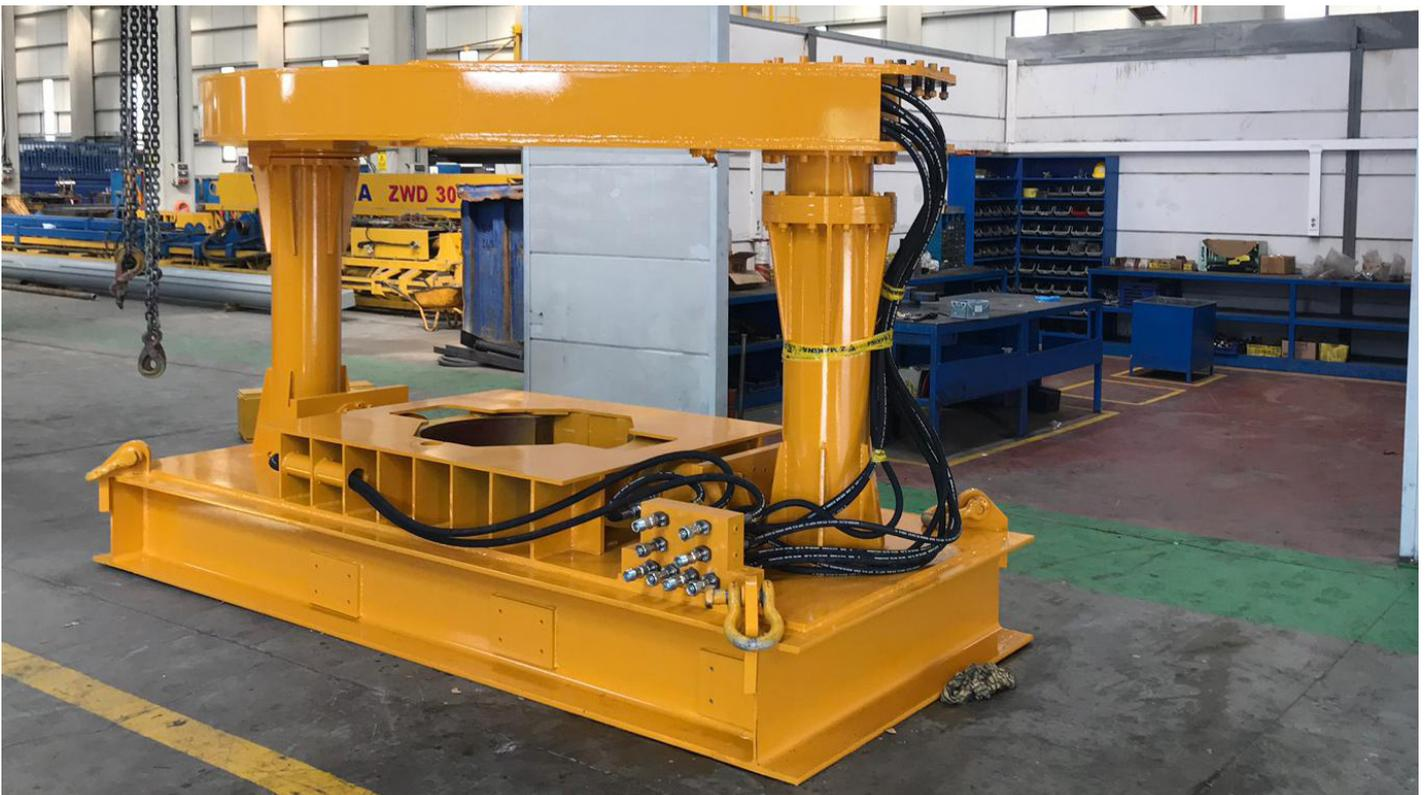
The installation of the conductor casings ranging from 20" to 30" diameter are installed by the Power Tong ZPT 30 with the torque needed to make up the conductor pipes is monitored, and controlled. According to the selected diameter of the casing, PLC system limits the tightening torque in order to avoid structural failures. In other words the make-up torque ratings rely on casing size, grade, metallurgy, weight, and the thread compound friction factor being utilized.
