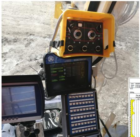
With Jean Lutz DATA Logger systems, Z Makina provides live streaming on job site, and data collection of operation.
