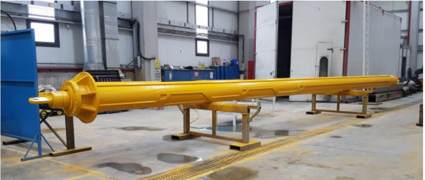
Kelly bar is the main part of a drilling machine, and the performance of the machines is affected by its quality. The fundamental goal of kelly bar is to transfer the maximum torque and pressure supplied by the drilling machine. Z MAKINA provides kelly bar for all types of rotary drilling rigs.
