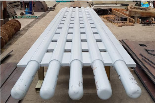
Stop-ends are easily placed to the ground and coupled together through special steel bars. They are made of sheet metal welded and internal pipes reinforcing the structure increasing its strength and toughness to prevent it from any damage. It is easy to connect or disconnect.
