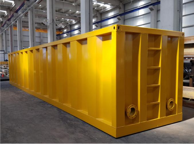
The bentonite tanks for bentonite muds and plastic mixtures are enormously strong that is stiffened oversized profiles, and electro-welded pressed steel sheet with the appropriate thickness.
