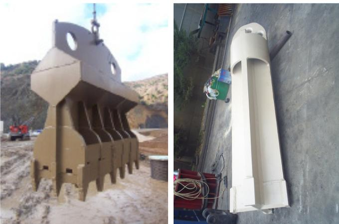
Z MAKINA Diaphragm wall and pile rig chisels penetrate rocks, boulders, and soil limitations to accelerate the grab excavation. Z MAKINA produces a broad selection of chisels in free-fall use to penetrate through the obstructions during excavation. Z MAKINA Chisels incorporate high-tensile, Hardox 500 steel and S 355 on the cutting edges to abrasion for resistance to wear and cold bending.
