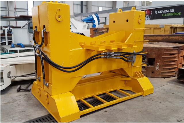
As soon as the concrete begins to set, extractors pull out the stop-end elements. Z MAKINA produces for the extraction of stop-end elements having a width from 500 to 1500 mm and pulling capacity up to 4000 kN. The system is complete with locking system pins to prevent dropping of the column. Z MAKINA supplies the hydraulic power pack for the extractors, customized for the adequate power. A remote control integrated with power pack to operate the unit is also available as optional.
