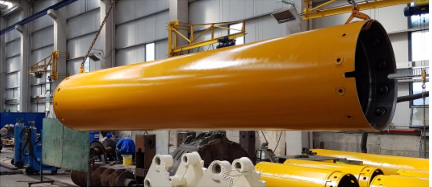
The Casings are used to protect the whole drilling operation; principally the rotary drilling tool during the operation, performs inside a mechanical protection executed by the casings fixed into the ground. Those casings are recovered for reuse.
