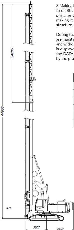
Z Makina has developed a jet grouting system with the single stroke columns to depths of 36 m capacity. It was designed which can be mounted on the piling rig used for jet grouting come in a range of different sizes; large ones, making it a perfect technique for improving the foundation of an existing structure.
