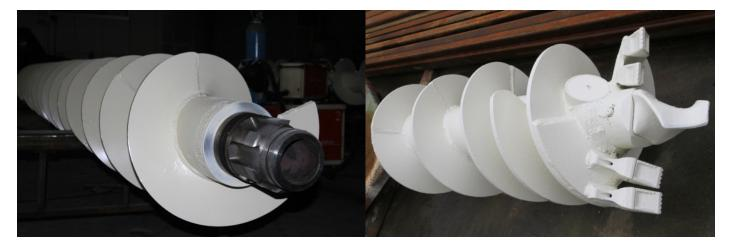
CFA piles are a type of drilled foundation in which the pile is drilled to the final depth in one continuous process using a CFA then concreting through the augers while extracting the tools.
